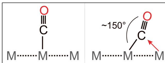
Figure 4.7: Schematic representation of on-top adsorbed carbonyl (left) turning into a semi-bridging carbonyl (right).
